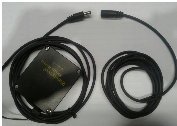
Fig. 18– Battery box connection
