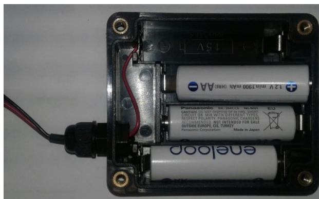
Fig. 21 – Replacing battery in battery box
