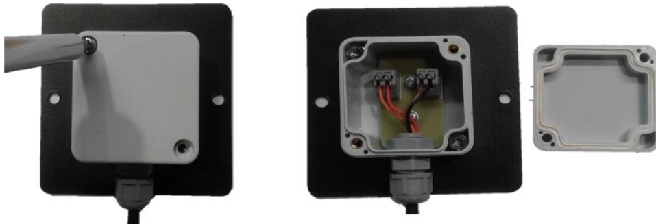
Fig. 13 – Opening the back of the wallswitch
