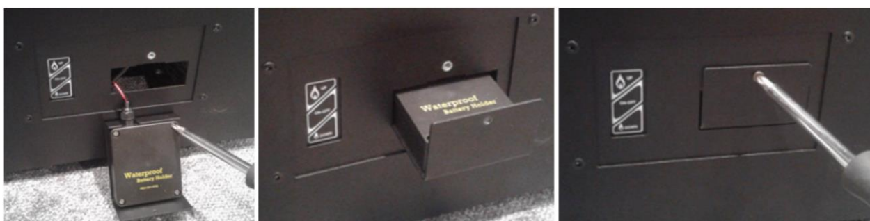
Replacing the batteries in the container
