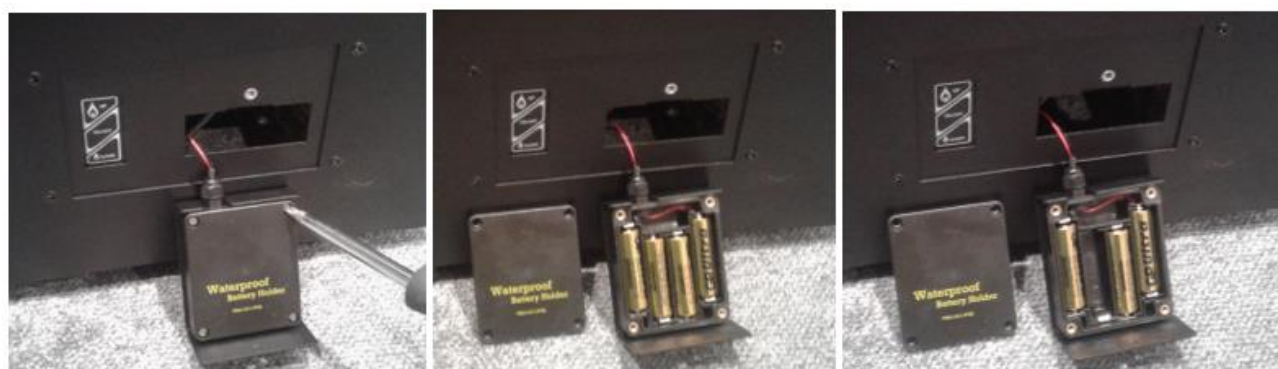
Replacing the batteries in the container
