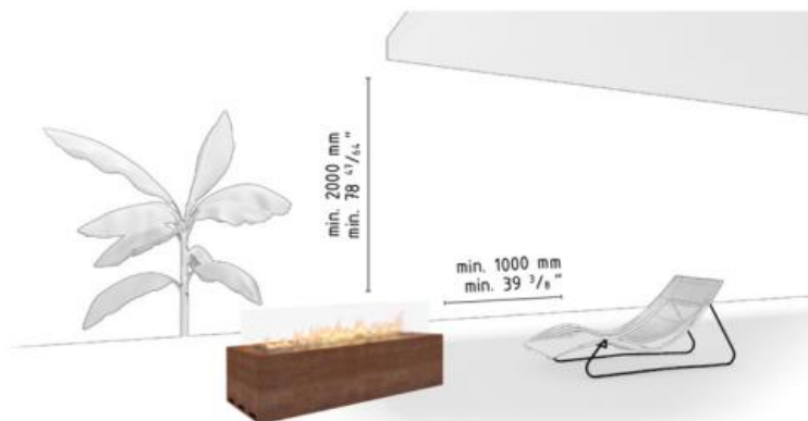
Fig. 1: Minimum distance to flammable materials
