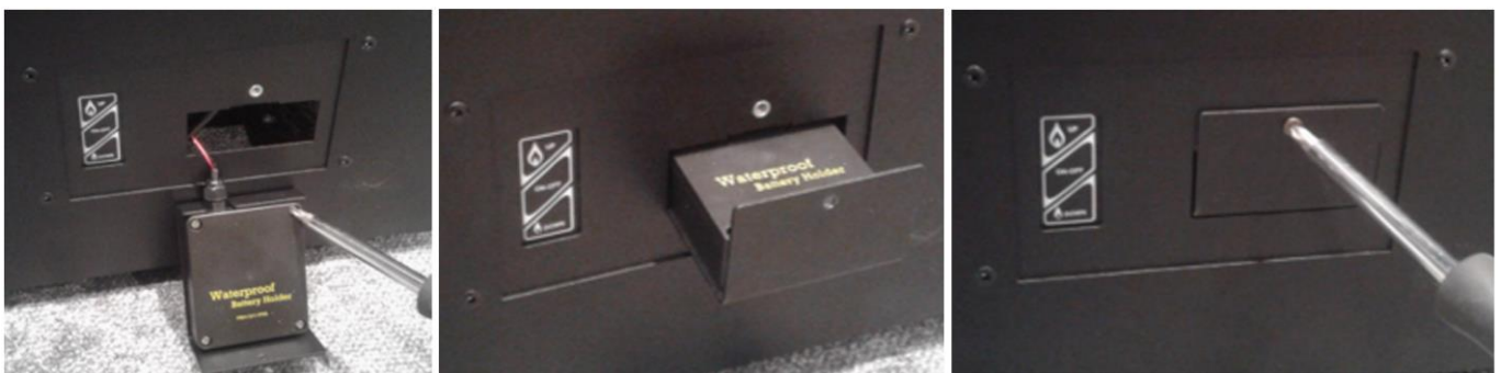
Fig. 11 – Putting back the battery box
