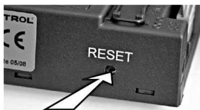
Fig. 7 – Receiver "RESET" button
