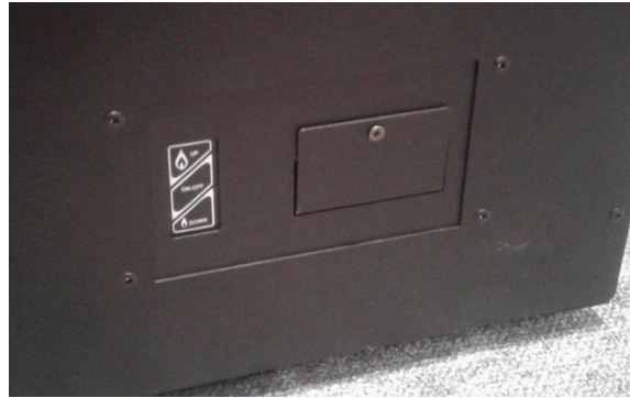
Fig. 8 – Receiver batteries containers
