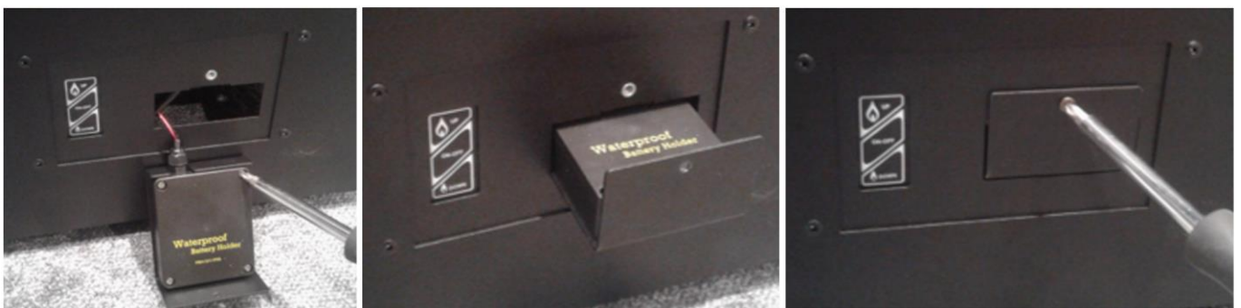
Fig. 11 – Putting back the battery box
